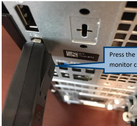
Press the locking tab to release the monitor cable from the port.
